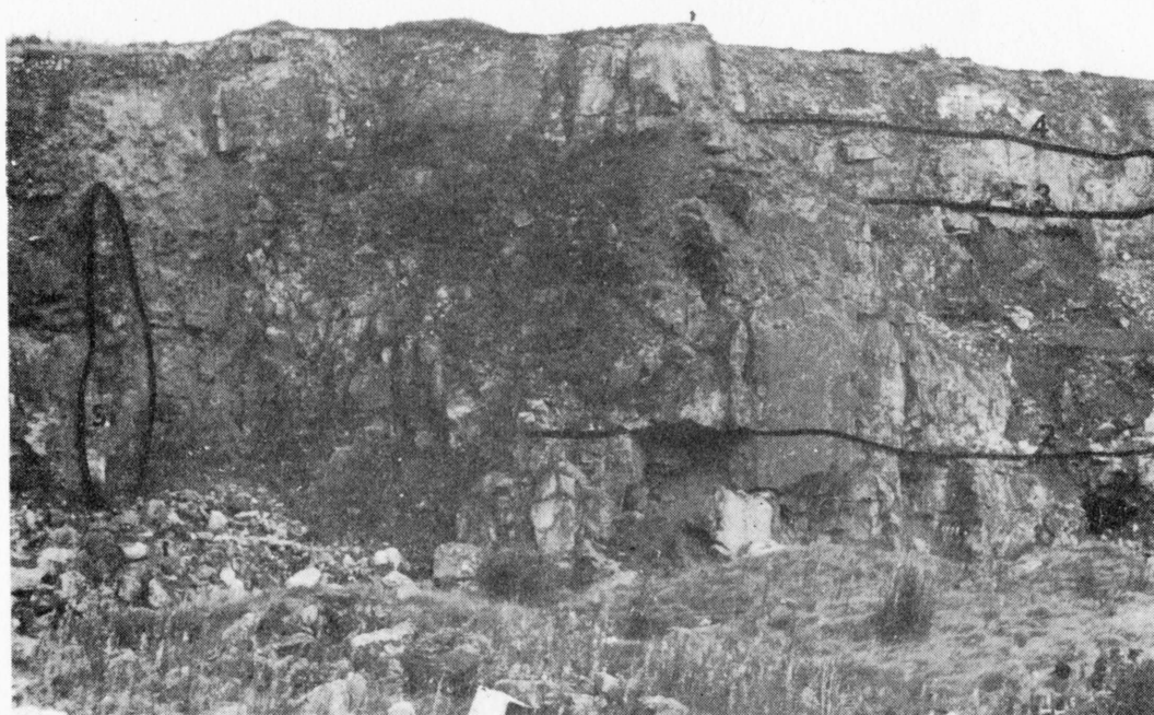
Fig.2. View of Masson Opencast Quarry looking north-east. Three clay wayboards (black lines) are present (2, 3 and 4) with their associated solution cavities (below wayboards 2 and 3). An isolated porcellenous limestone raft can be seen (just above wayboard 4). A prominent silicified limestone-dolomite rib can be seen on the left of the photograph (labelled Si).
